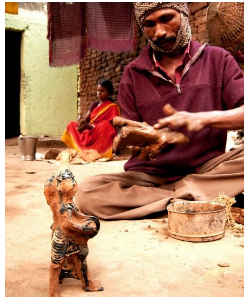
Picture 7: Artisan pasting clay over the (black) wax replica. Bikna Dokra Village, Bankura, West Bengal, India
